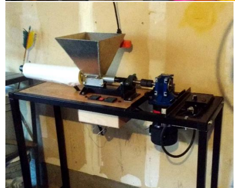
Above: Tyler Linner holding pelleted plastic from broken sleds for repurposing. Below: The Precious Plastics extruder.
