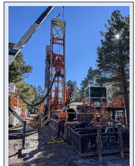
This specialized dual rotary rig effectively seals off any cracks or caverns encountered along the way and does not require the circulation of drilling water.
